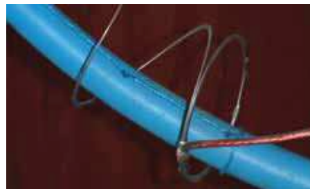
PHOTO 2: Detail of how the Slinky is mounted on the water pipe. The string is tied to the Slinky on the hidden side of the pipe.
