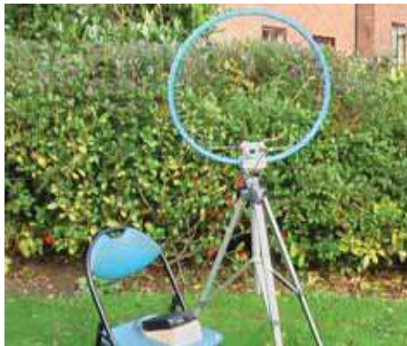
PHOTO 1: The completed Slinky loop antenna, mounted on a tripod.
