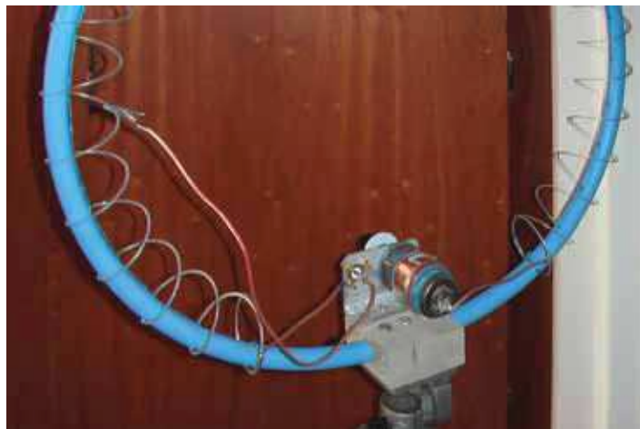
PHOTO 3: General view of the business end of the loop, showing the mounting block, capacitor/input socket bracket, wiring and my tapping point.
